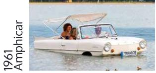
Despite what we all saw in The Jetsons, flying cars that can fly are a long way off. In 1961, however, you could have a car that was also a boat. The 1961 Amphicar featured a pair of propellers that could provide a cruising speed of up to seven knots.
